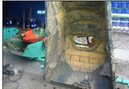
Rubber and tile lined chute after 1,500 hours
