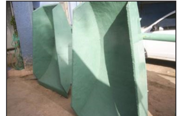
ARC BX1* coated chutes with ARC S2 topcoat
